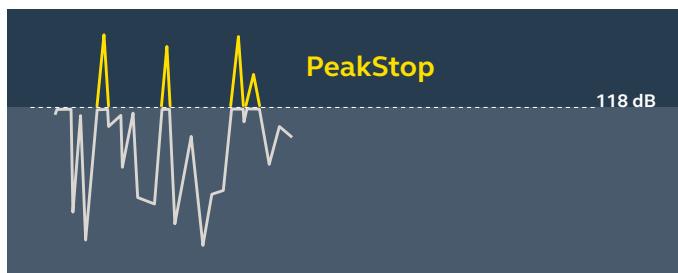
Fig. 2: PeakStop continuously monitors the sound flow and actively reduces critical sound peaks to a safe level.
